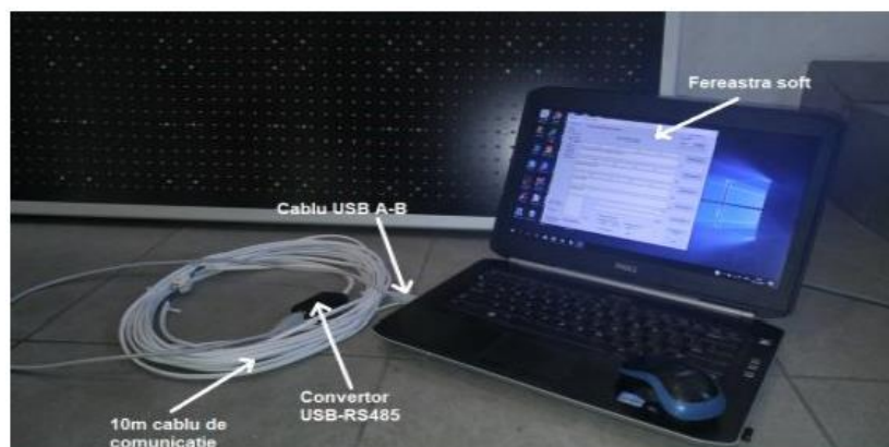
Figure 5. Programmable LED display and its programming possibility
